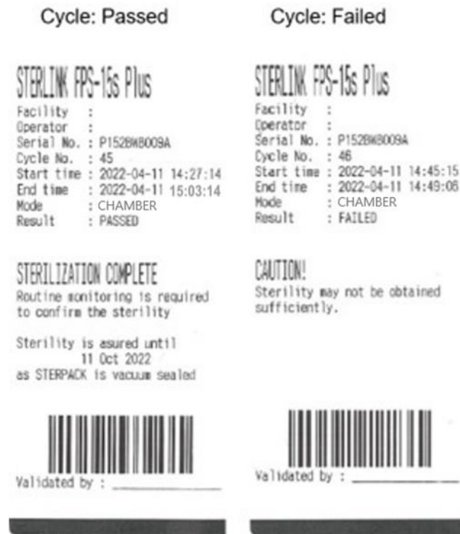
Fig. 7.2 Short format report for passed and failed cycle
